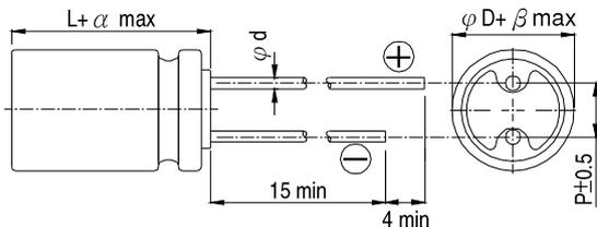
LEAD SPACING AND DIAMETER Unit: mm
